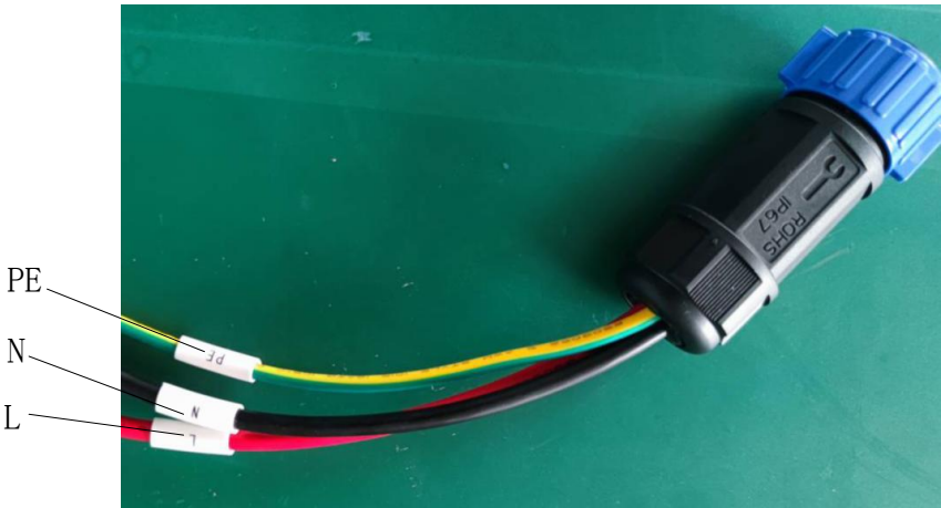
Figure 6-4 ACIN connector line sequence nameplate schematic
